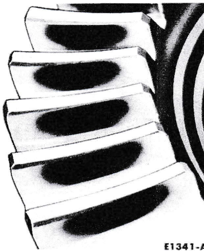
FIG. 8—Acceptable Non-Hunting Pattern—Uniform
