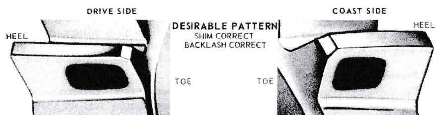
FIG. 2—Ideal Tooth Pattern—Integral Carrier Type Axle
