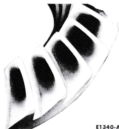
FIG. 7—Acceptable Non-Hunting Gear Set—Coast Pattern
